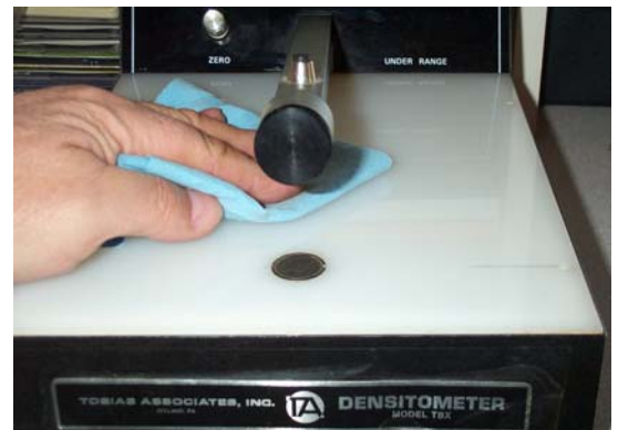
Clean with a lint free cloth lightly dampened with water
