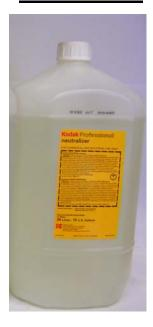
Mix at 18-32C or 65-90F Start with 875ml of water, add 125ml of neutralizer concentrate, and then mix until the solution is uniform.
